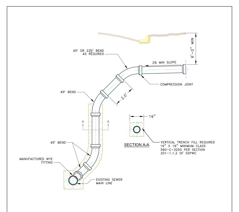
NOTE 1: CHIMNEY SERVICE LATERALS SHALL BE INSTALLED ON ALL LINES 15' DEEP OR GREATER
