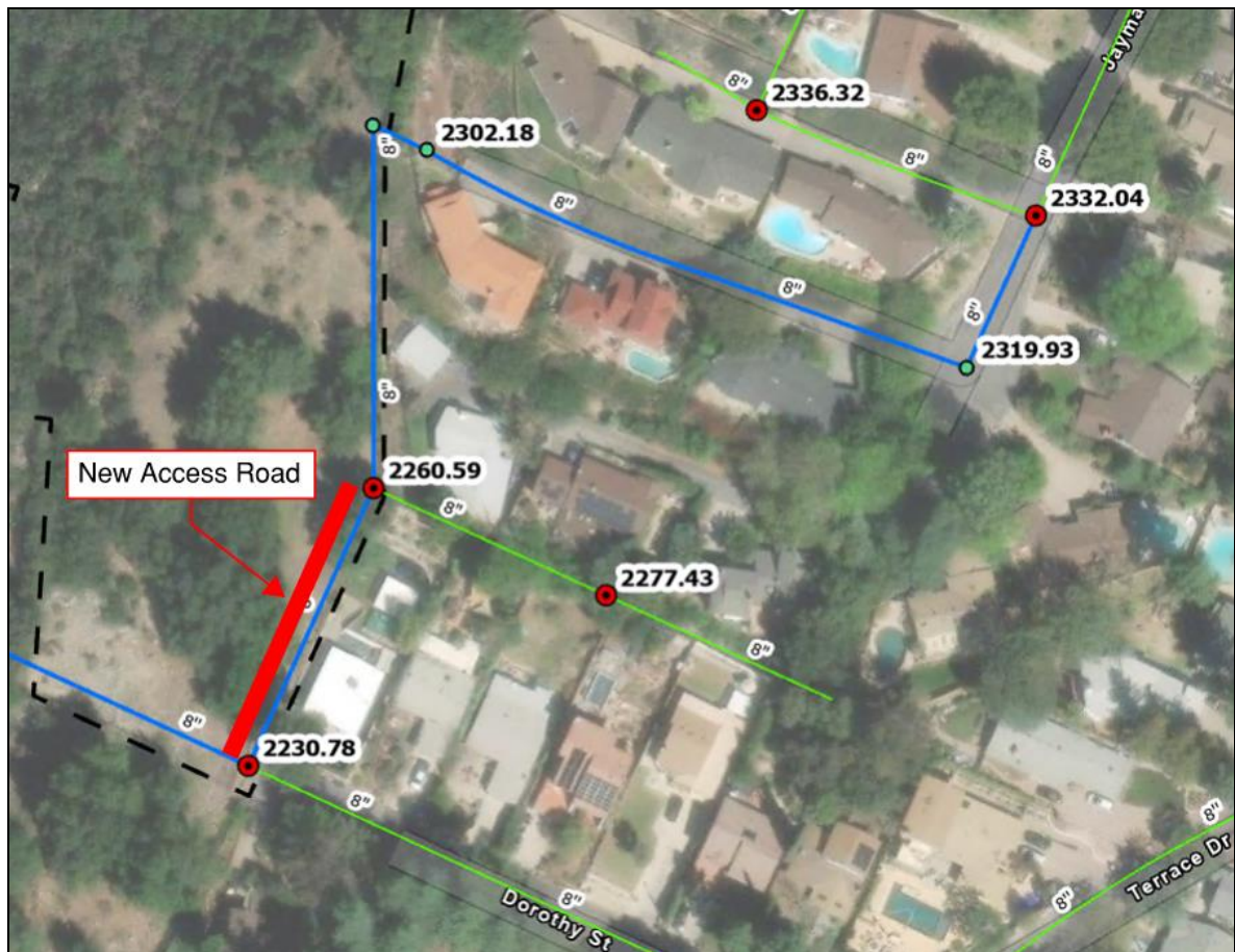
Figure 7: Dorothy / Goss Canyon Access Road
