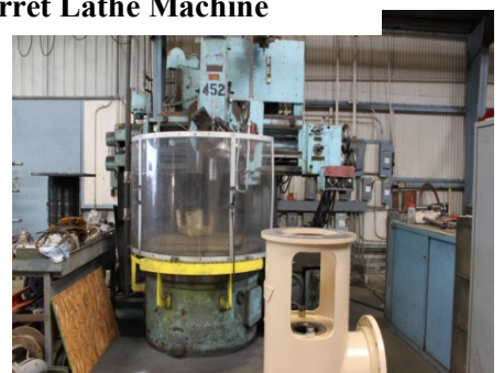
Vertical Turret Lathe Machine
